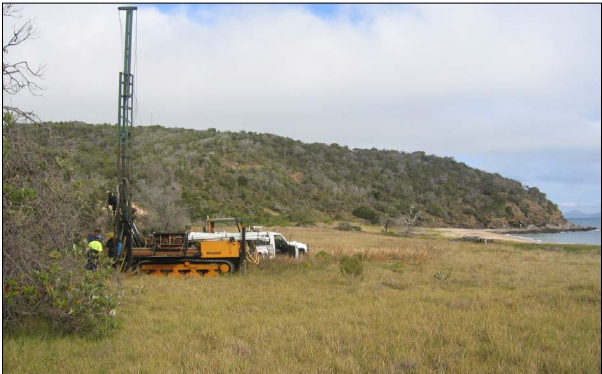
Photo 2: Drill rig set up on Monitoring Bore 3, near Butterfish Bay, Northeast Aquifer.
